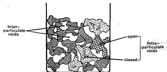
FIG. 4-4. Diagram of various intraparticulate and interparticulate air spaces in a bed of powder.
